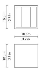
Wall lamp with a matt white or dark grey painted die-cast aluminium frame and a transparent polycarbonate diffuser. The high IP rating (IP54) makes the lamp ideal for indoor and outdoor use. It has independent control of the beam of light above and below.
