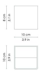
Wall lamps with a matt white or sand painted die-cast aluminium frame and a transparent polycarbonate diffuser. The product is suitable for indoor use only.
